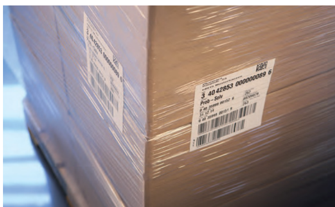
Industry: Retail / Distribution Application: Pallet labelling to GS1 Standard
