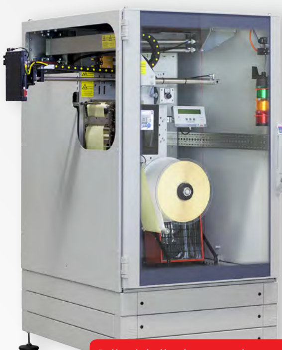
Pallet labeller in protective enclosure with built-in heating system
