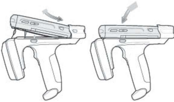
Slide the mobile computer into the Sled until it locks into place. The latches secure the mobile computer to the sled.
