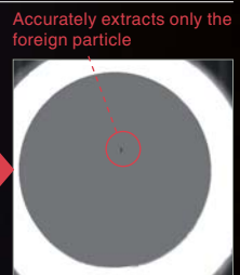
Particle detection on backgrounds with glare and other shade variations
