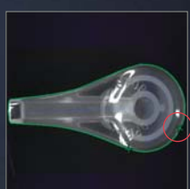
Detection of minute flaws along the profile
