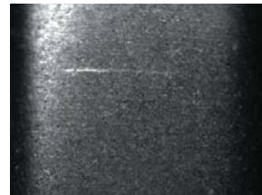
The same workpiece with a line-like scratch.
