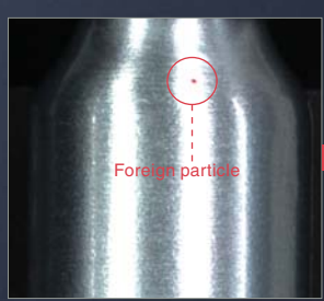
Foreign particle detection on a rounded metal surface
