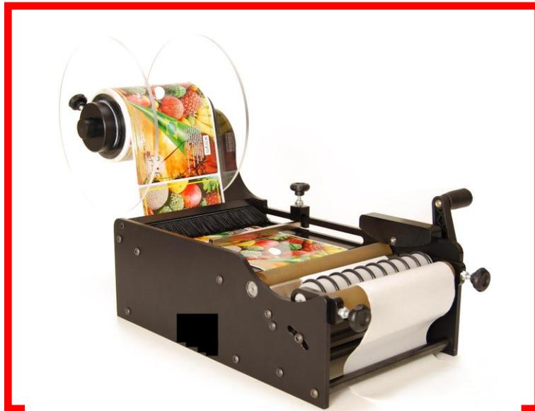
The NEW MBA01 is a manual applicator ideal for short and low volume applications and has been developed to apply labels to a wide range of cylindrical containers including Bottles, Jars, Cans, Tubs and Tubes.
